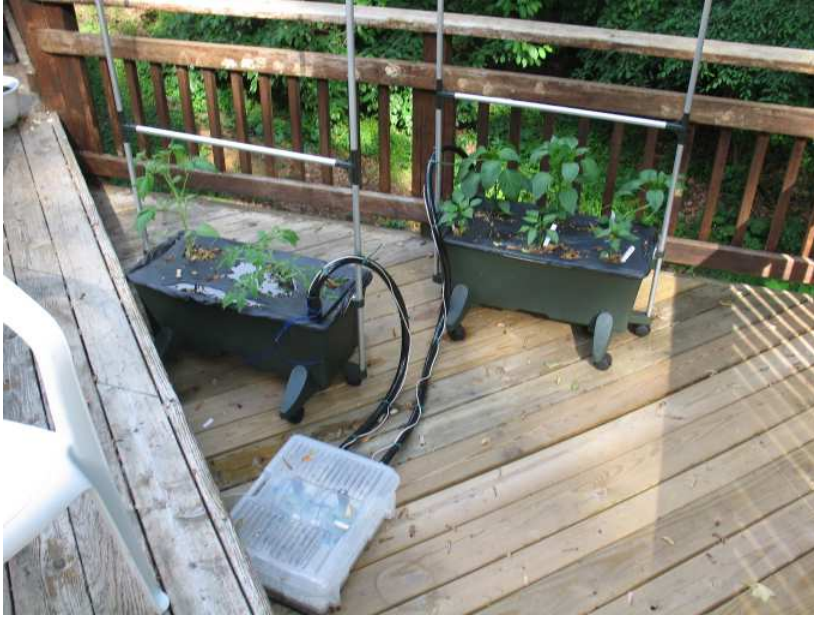
Figure 4 Photo of single Remote Box is shown connected to Earthboxes. The Remote box supplies water to each Earthbox through the black hoses. The remote box contains an internal water proof box for the electronics as well as the PVC manifold and valves. The water sensor wires are the white wires coupled to the hose and feeding back to the remote box.
