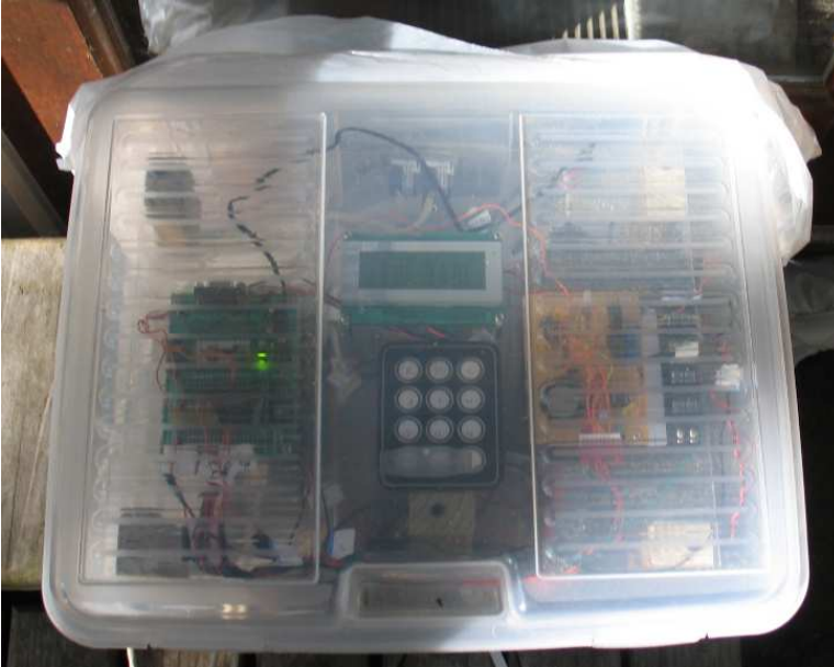
Figure 3 Photo of Controller Box. All components are visible. In center is LCD display and Keypad; Javelin Stamp is located on the right. RJ45 connections are to rear of box. A dual color leds flashes to indicate overall status of the system. It is green indicating proper operation (other wise it would flash red)
